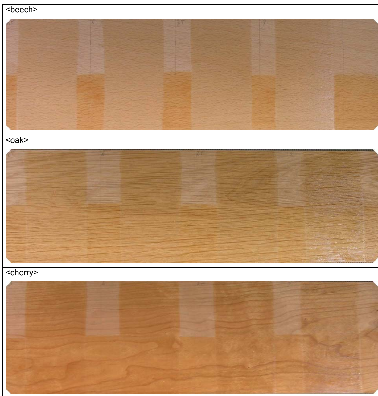
Figure 1. Panels change of pH, topdown beech panel, oak panel and cherry panel.
